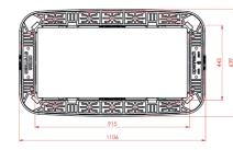
Typical depth Cubis Internal Depth per Weight per Product Dimensions section of chamber section **Product Code** 10901300 JMF 102 725mm x 255mm 150mm 600mm 5.8kg JMF 104 915mm x 445mm 10.9kg 10901301 150mm 600mm 10901302 JMF 106 1310mm x 610mm 150mm 750mm 16.2kg
