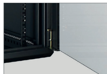
The L-shaped spring pin allows for quick installation of the front door, and offers the possibility of changing the opening direction quickly.
