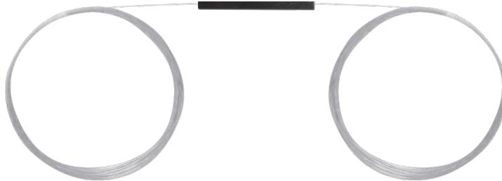
The 2xN splitters perform the same function as 1xN splitters, except that the coupling is made with two input fibers instead of one. This provides a test port in an installation without having to disconnect and interrupt the traffic on the line.
