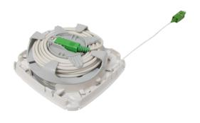
The eline® extension box is a small unwinder reel with 40m of discreet optical cable (Ø 0.9mm) on one side and 3m of 3mm cable on the other side. Both sides are SC/APC preconnectorised.
