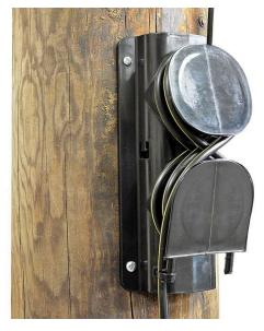
The Fibre Locking Device (FLD) provides an effective solution that isolates the termination of the fibres, both spliced and connectorised in the fibre enclosure from 'in span' environmental loads such as ice and wind.
