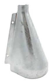
The Connector Bend No.1 is essential for seamlessly connecting ducts to Capping Steel at distribution points. Specifically designed for 90mm ducts to 19mm connections, it ensures efficient and reliable distribution of cables in various applications.
