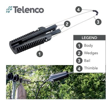
The ACADSS clamps are used for the anchoring of 9mm to 19mm aerial round ADSS cables on distribution networks. They are to be installed on poles or facades where spans do not exceed 90m.
