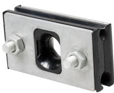
The Telenco® SC37C and SC711C suspension clamps are designed to provide an articulated suspension for figure-8 cables with steel or dielectric insulated messenger on access network with spans up to 90m. Its unique patented design has been developed to offer an universal hardware fitting covering all suspension cases on wooden, metal or concrete poles. With straight grooves and a reversible system, these clamps are compatible with messengers diameters from 3 to 7mm and 7 to 11mm.
