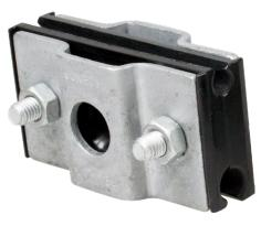
The Telenco® SC39B suspension clamp is designed to provide a **fixed** suspension for figure-8 cables with steel or dielectric insulated messenger on access networks where spans do not exceed 70m.
